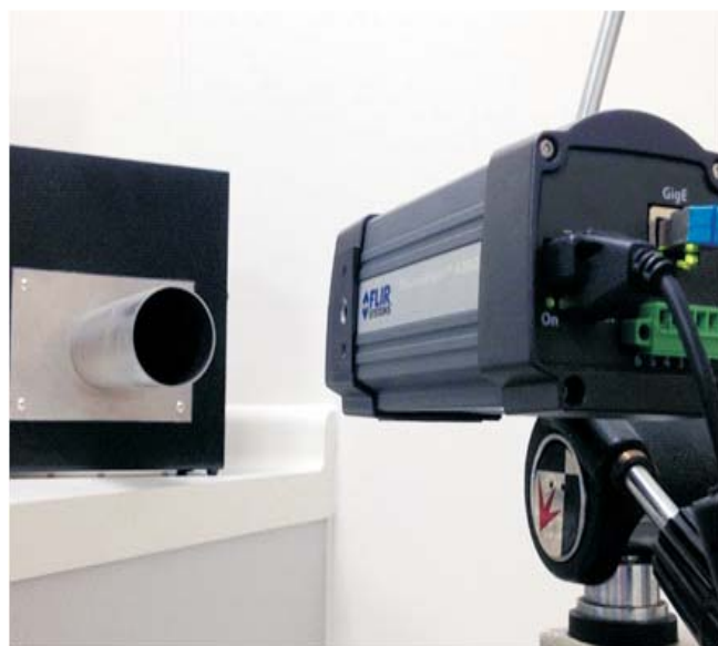
Figure 1: Picture of the set up used when imaging the blackbody source
