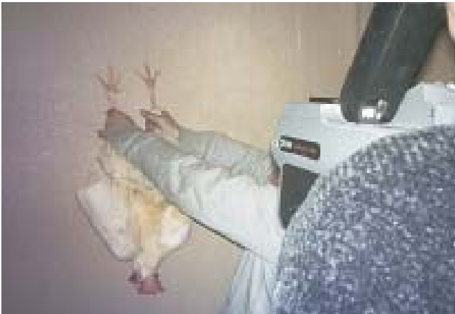
Figure 1 Using a FLIR ThermoCAM®™ PM695, thermal images of the ventral view of the foot were taken at 0.91 meters from each selected hen
