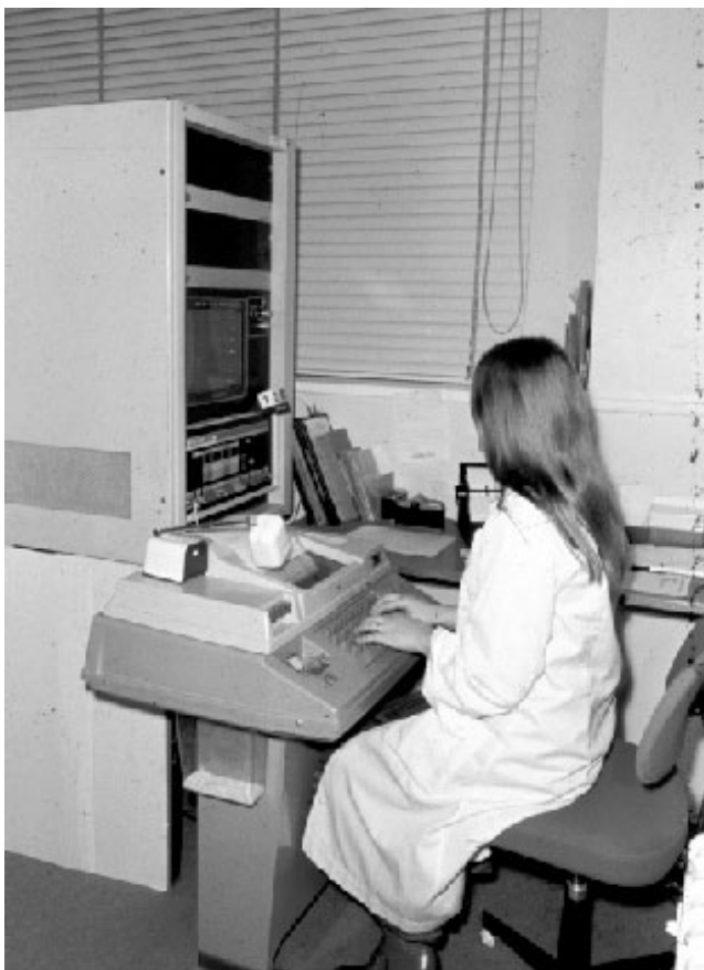
Figure 4 Pdp8e computer with teleprinter terminal used in Bath 1973 adapted from a Swedish nuclear medicine system
